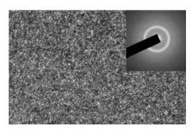
TEM image of co-sputtered cathode LSC113 -50 % LSC214. Note that in co-sputtered state the cathode is amorphous (Sari et al, 2018)
