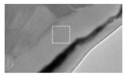
TEM image of a portion of symmetric cell with LSC113 -50 % LSC214 cathode. Granular region is electrolyte and dotted square shows a portion of a cathode where SAD is taken (Sari et al, 2018)
