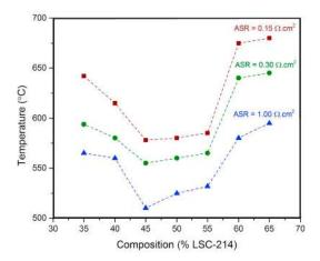
Variation of temperature where ASR= 0.15, 0.30 and 1.0  $\,\Omega$  cm2 with composition. Note that temperature is minimum at LSC113- 45%LSC214. (Sari et al 20018)
