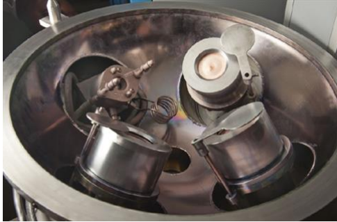
Magnetron sputtering with three guns used in combinatorial development
