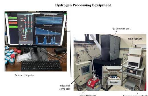
*Equipment used for hydrogen processing of the turnings. The reactor where turnings are treated is inside the split furnace. The equipment is a PCT apparatus (house built and improved over a period of 10 years) adapted for the purpose*
