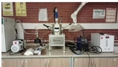
Figure 1. Arc Melter System
